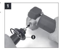
Prepare a proper 4" backing pad (not provided) and screw tight with hand onto the male threads of the work spindle (G) while holding the wrench (J) on the flats of the spindle. (See Figure 2)
