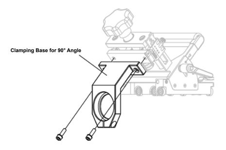
3. Attach 90° Clamping Base to Main Base.
