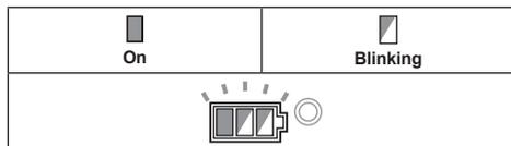
If the tool does not start, the battery may be overheated. In this situation, let the battery cool before starting the tool again.
